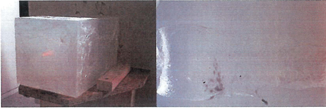
Figure 5: Soap block at 10 m in front of test machine rifle (laser shows the point of aim) and a sample picture of a cavity produced inside the block by a passing projectile.
